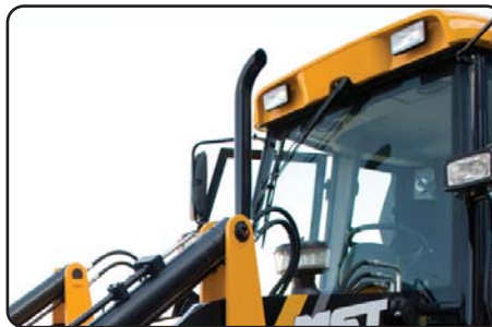
14.5 litres of muffler capacity. Reinforced flexible exhaust, venturi system outlet pipe mounted on the frame independently of the muffler. Trouble-free operation at temperatures up to 60°C thanks to the new venturi system throwing out the engine heat.
