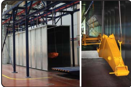
Totally enclosed paint spraying booth which is protected against external factors and longer than a soccer pitch, where every part including the frame can be painted
