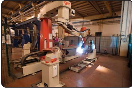
Defect-free welding technique thanks to robot welding having 3-D processing capacity
