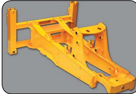
One-piece (I) heavy-duty frame, processed with unrivalled 3-D Robot Welding technique
