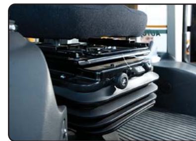
Antiperspirant operator seat the height of which can be adjusted according to the operator's weight and by means of compressor air
