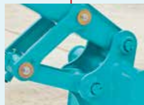
Bucket Cast-iron idler link provide greater strength.
