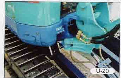
Grease four times at each 90 degree position of upper frame.
