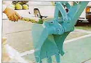
Greasing swing bracket pin bushing.
