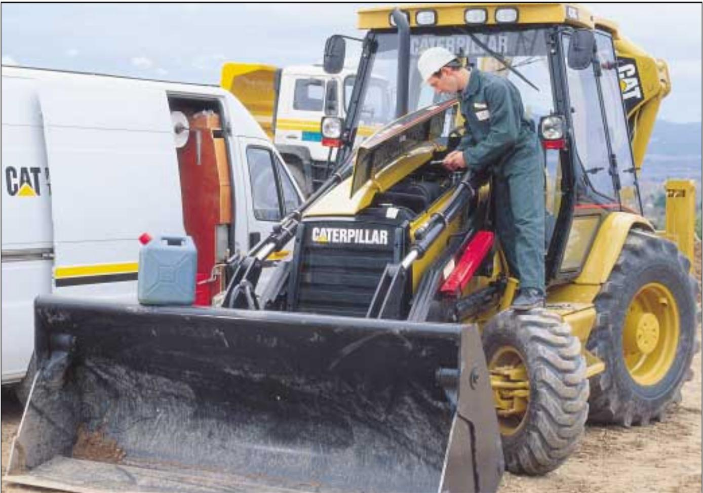
**Quick, Easy Access.** All daily fluid servicing is done on the left side of the machine. A flip-open engine hood with pneumatically-assisted lift cylinders provides convenient access to a single location for fluid level checks. Visual indicators make it fast and easy to check air cleaner and hydraulic oil level. All filters are mounted vertically for spill-free servicing.
