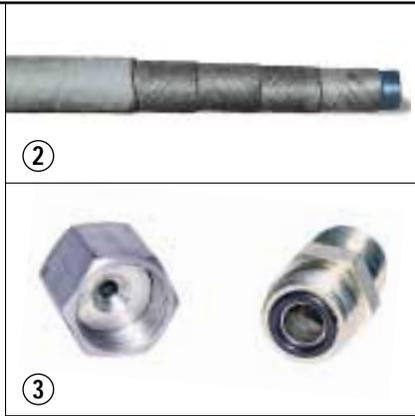
**Caterpillar XT hoses** are used for high pressure applications to substantially reduce downtime from hose failure. The Cat XT-3 hose is made of four overlapping, insulated wire spiral wraps bonded together for unrivaled long life. XT-3 hoses exceed SAE certification standards, and the hose routing protects them from work damage. If a hose does need replacing, it's fast, easy, and requires no special tools.
